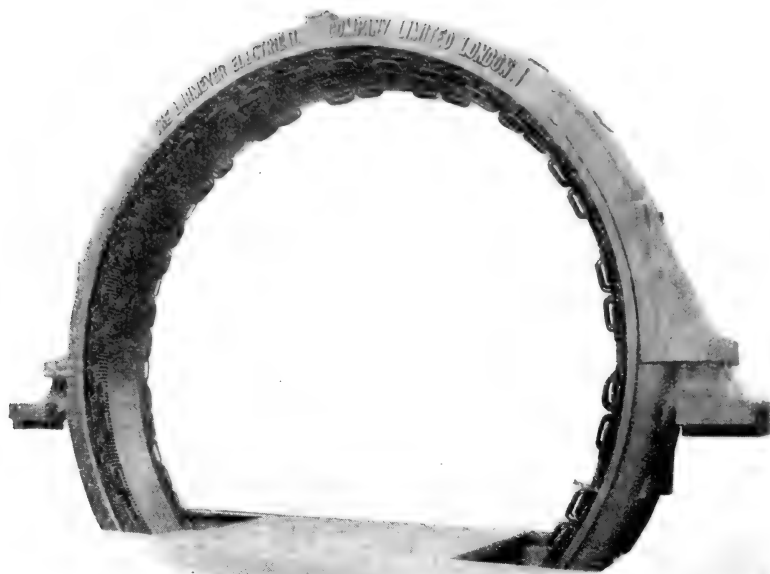
FIG. 255.—Armature of Lahmeyer 4000 k.w. 10,000-volt Alternator. Thirty-six-pole, Three-phase, Whole-coiled, Double-coil, Four-slot Spiral Winding in three ranges.
